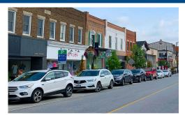
On-street parking is the reduction of roadway width available for vehicle movement by allowing motor vehicles to park adjacent and parallel to the curb.
