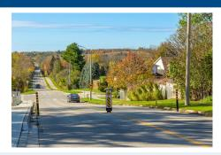
Flexible post mounted delineators are used to create the effect of a median, thus giving a sense of constriction for drivers.
