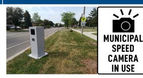
Automated Speed Enforcement (ASE) uses a camera and a speed measuring device to detect vehicles travelling in excess of the posted speed limit and capture its image as proof for conviction.
