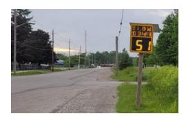
A speed display device is an interactive sign that displays vehicle speeds as oncoming motorists approach. Vehicle speed is captured using radar and can trigger the display board to show when vehicle approach at predetermined unsafe speed.
