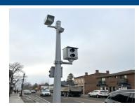
A Red Light Camera (RLC) is a camera that captures an image of a vehicle which has entered an intersection despite the traffic signal indicating red.
